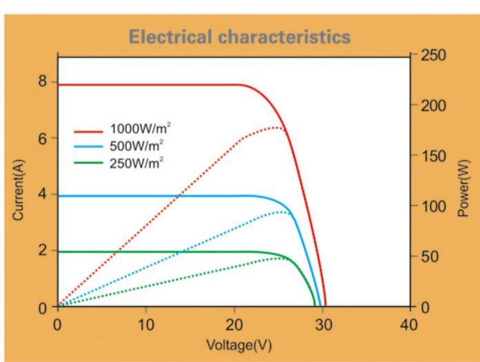
At STC( Standard Test Conditions).1000W/m, 25° C cell temperature, AM1.5 spectrum
